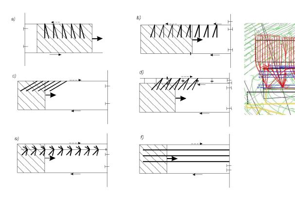
Drainage holes deployment in the area of longwall excavation
